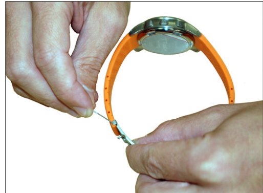
Step 3A: Use a push device, such as a small paper clip on the 6 o'clock side of the watch, and insert it into the hole where the spring bar sits connecting the strap and the buckle. It is important to remove the initial section(s) from the strap section on the 6:00 side of the watch.
