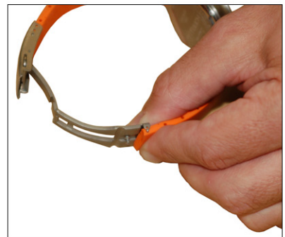
Step 9: Position the bottom end of the spring bar into the hole of the clasp and then position the top end evenly with clasp section.
