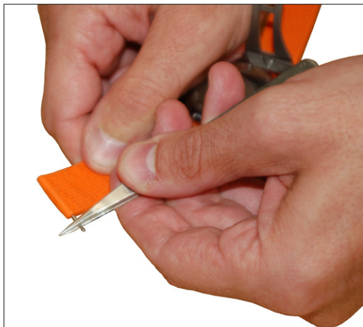
Step 5: Use a tweezer or plier to remove the spring bar from the strap. Take care to not pull the spring bar out by the end, grasp the piece as close to the center as possible.
