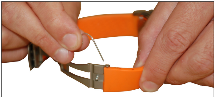
Step 10: Use your pushing tool (i.e. push pin) to push the top end of the spring bar and position it into the top hole of the clasp.
