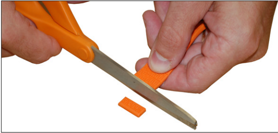
Step 7: Cut all the way through the strap section to be removed in a clean straight line.
