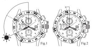
The Engineer Hydrocarbon Spacemaster Orbital (DC2036) can be used as a compass synched to the Sun or to store relative position with a separate compass.
